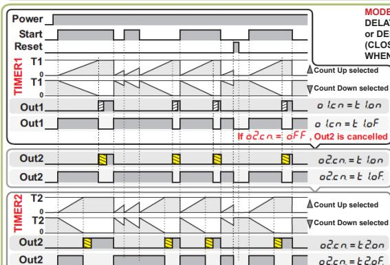
If  $o1ot$  or  $o2ot$  is set to HOLD, the output is continuous until the power is removed from the timer or the START input or RESET input is switched.
