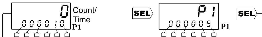
Press SEL, then use the Digit buttons to change P1. The display will flash. Press SEL again to accept the new value. If SEL is not pressed within 30 seconds of the last change, P1 will revert to the original value.
