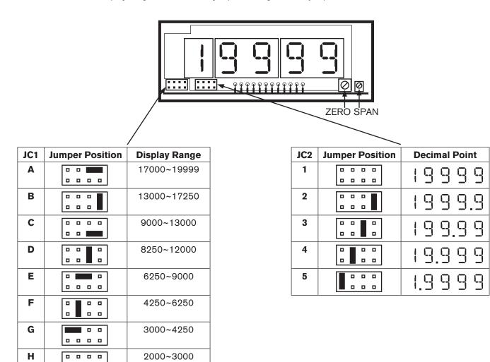
3. Connect the auxiliary power supply to the panel meter and switch on for at least 3 minutes.
