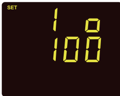
Fig 3-3 Full range shunt setting
