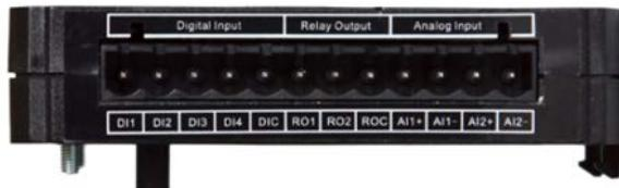
Figure 5-4 AXM-IO3 Module
