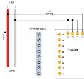
Figure 2-35b 1 Element 2 Wire (1LN-1CT) Configuration Using 333mV/mA CTs
