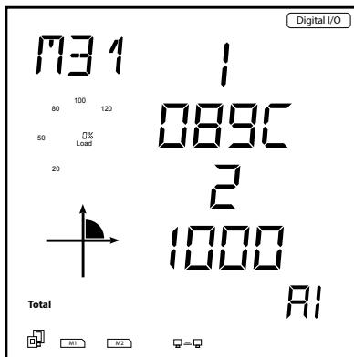
**Figure 5-42 Analog Input Reading from the Meter's Display**
