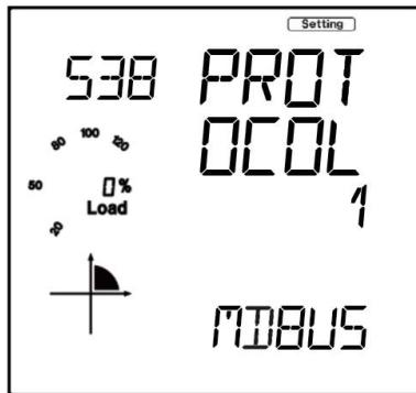
Figure 6-4 System Parameter Setting – S38 Protocol 1
