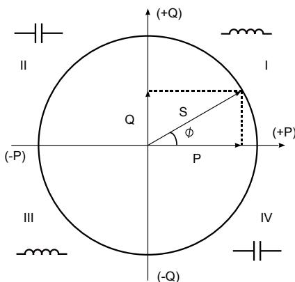
Figure 4-10 Four Quadrant Load Type and Power
