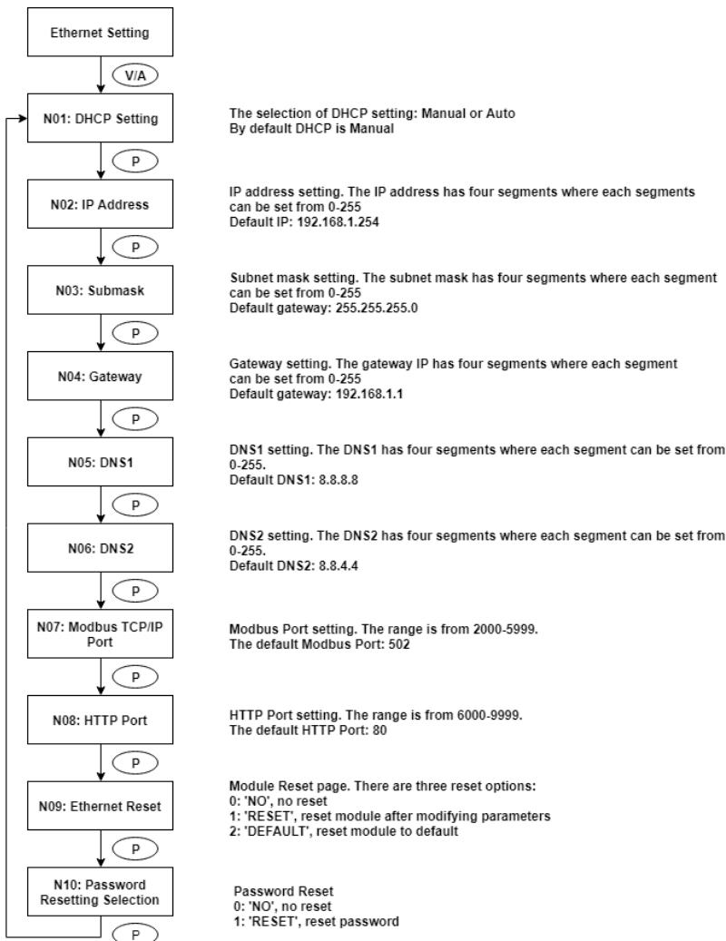
Figure 3-38 Ethernet Module Net Settings Screen Sequence
