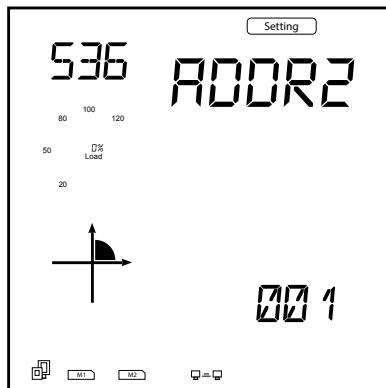
Figure 5-56 Address Setting for AXM-RS485
