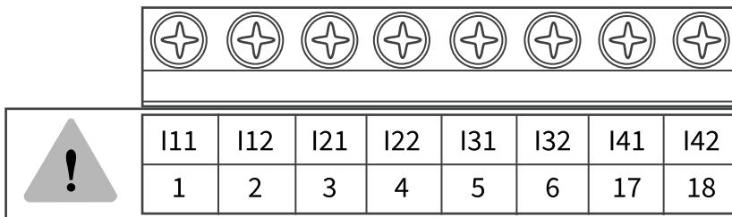
Figure 2-22 Current Input Terminal
