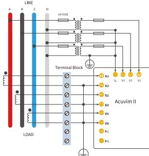
Figure 2-28a 3 Element 4 Wire Wye (3LN-3CT) Configuration with PTs Using 5A/1A CTs
