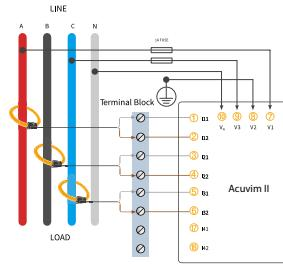
Figure 2-30c 2 1/2 Element 4 Wire Wye (3LN2.5 -3CT) Wiring Using Rogowski Coils
