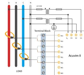
Figure 2-31c 2 ½ Element 4 Wire Wye (3LN2.5 -3CT) with PTs Using Rogowsky Coils
