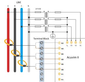
Figure 2-28c 3LN-3CT Configuration with PTs Using Rogowski Coils
