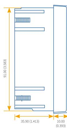
Figure 2-4 Side View of Remote Display Unit
