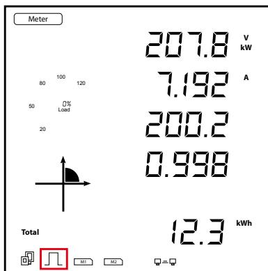
Figure 5-33 Pulse Signal Indicator on Meter's Display
