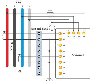
Figure 2-30a 2 1/2 Element 4 Wire Wye (3LN2.5 -3CT) Wiring Using 5A/1A CTs
