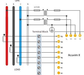
Figure 2-31b 2 ½ Element 4 Wire Wye (3LN2.5 -3CT) with PTs Using 333mV CTs
