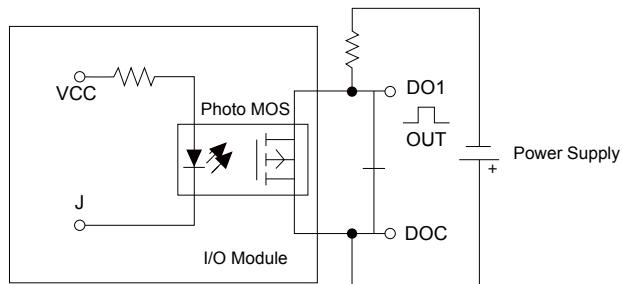
Figure 5-14 Digital Output Circuit
