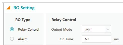
Figure 5-29 Relay Output Configuration from Acuvim 2 Software
