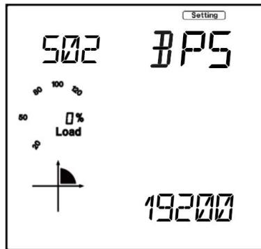
Figure 6-3 System Parameter Setting - S02 Baud Rate
