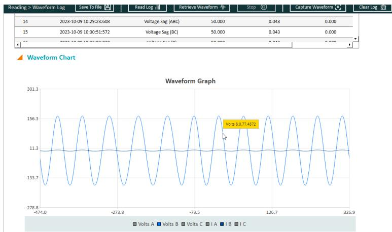
Figure 4-49 Retrieve Waveform Phase B Voltage and Current
