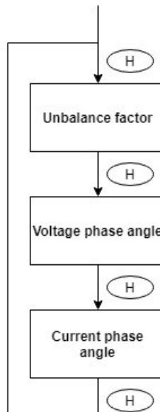
Figure 3-9 Phase Angle and Unbalance Screen Sequence
