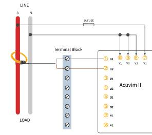
Figure 2-35c 1 Element 2 Wire (1LN-1CT) Configuration Using Rogowski Coils
