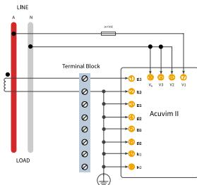
Figure 2-35a 1 Element 2 Wire (1LN-1CT) Configuration Using 5A/1A CTs
