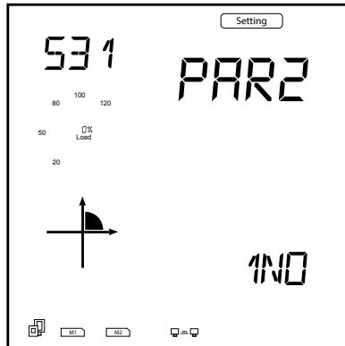
Figure 5-55 Parity Setting for the AXM-RS485 Module
