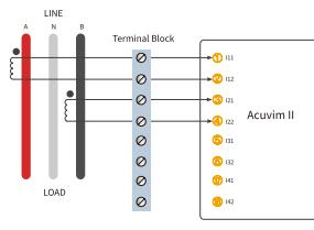
Figure 2-25b 2CT Wiring for 333mV/mA CTs in 1LL Split-Phase Systems
