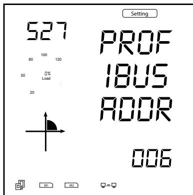
Figure 5-51 AXM-PROFI Address Setting on Meter's Display
