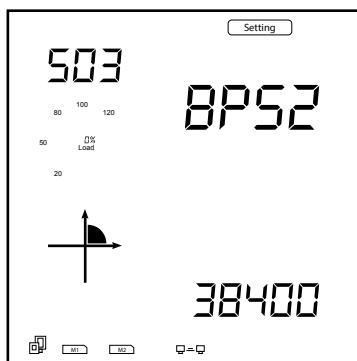
Figure 5-54 Baud Rate Setting for the AXM-RS485 Module
