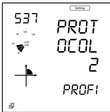
Figure 5-50 Protocol 2 Setting on Meter's Display
