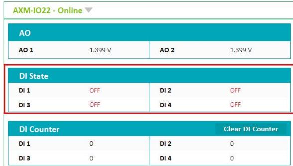
Figure 5-21 Digital Input Status Readings from the Acuvview 2 Software
