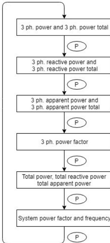
Figure 3-6 Power, Power Factor, and Frequency Screen Sequence
