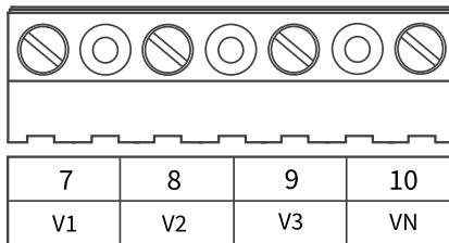
Figure 2-20 Voltage Input
