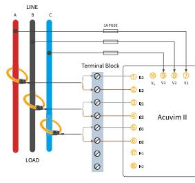
Figure 2-29c 3 Element 4 Wire Delta (3LL-3CT) Configuration Using Rogowski Coils
