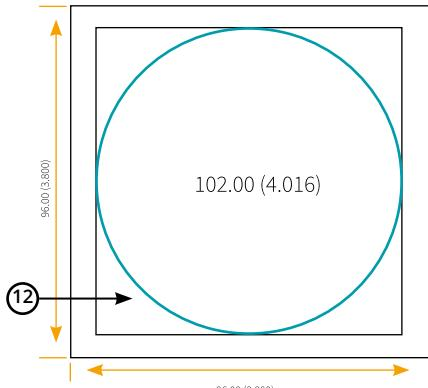
Figure 2-2 Rubber Gasket
