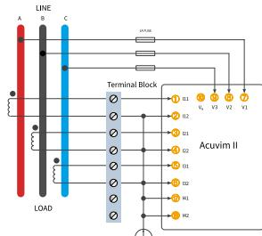
Figure 2-29a 3 Element 4 Wire Delta (3LL-3CT) Configuration Using 5A/1A CTs
