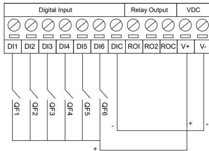
Figure 5-11 Multiple Channel Digital Input Wiring Using 24Vdc on AXM-IO1 Module
