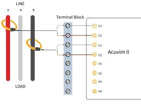
Figure 2-25c 2CT Wiring for Rogowski Coil (RCT) in 1LL Split-Phase Systems
