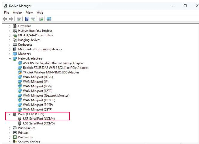
Figure 4-2 COM Port Number Assigned to USB Converter
