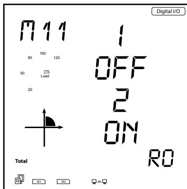
Figure 5-28 Relay Output Status Readings
