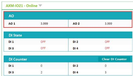
Figure 5-41 Analog Output Readings on the Acuvim 2 Software
