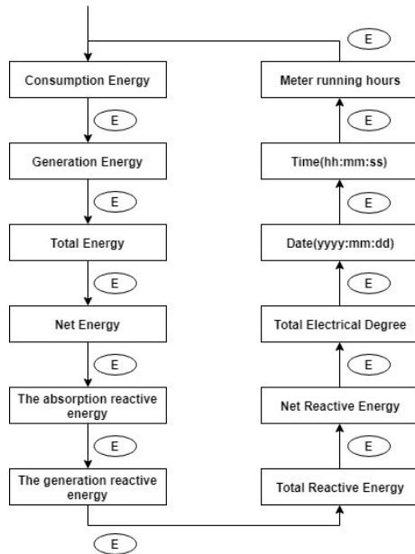
Figure 3-12 Energy and Real Time Clock Screen Sequence
