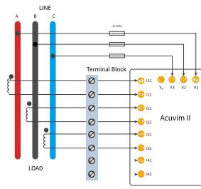
Figure 2-29b 3 Element 4 Wire Delta (3LL-3CT) Configuration Using 333mV/mA CTs
