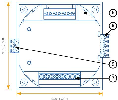
Figure 2-6 Rear View of Acuvim II Meter
