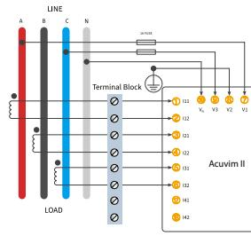
Figure 2-30b 2 1/2 Element 4 Wire Wye (3LN2.5 -3CT) Wiring Using 333mV CTs
