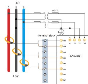
Figure 2-32c 2 Element 3 Wire Delta (2LL-3CT) Wiring with PTs Using Rogowsky Coils
