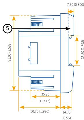
Figure 2-5 Side View of DIN Rail Meter
