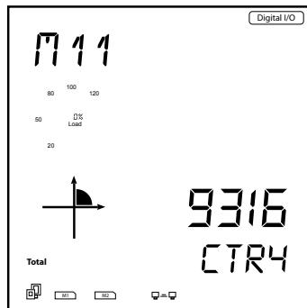
Figure 5-24 Digital Input Pulse Count from Meter's Display
