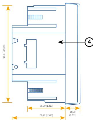
Figure 2-3 Side View of Meter With Display
