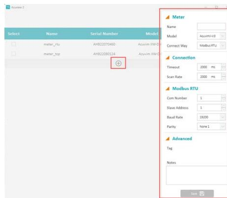
Figure 4-3 Creating New Connection Using the Acuvim 2 Software
