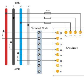
Figure 2-27b 3 Element 4 Wire (3LN-3CT) Wiring Using 333mV/mA CTs
