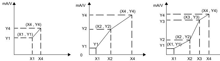
Figure 5-40 Relationship Between Analog Output and Electrical Parameters
