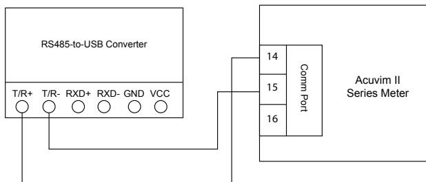
Figure 4-1 RS485-USB Converter Connection to Acuvim II Meter
