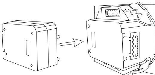
Figure 5-48 AXM-PROFI Installation to Acuvim II Meter
