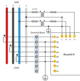
Figure 2-31a 2 ½ Element 4 Wire Wye (3LN2.5 -3CT) with PTs Using 5A/1A CTs
