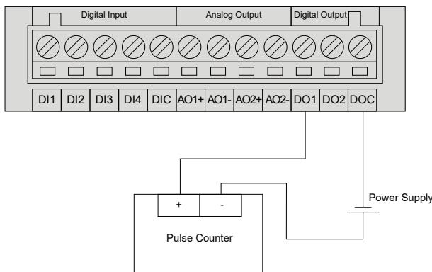
Figure 5-16 Digital Output to a Pulse Counter
