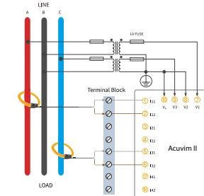
Figure 2-33c 2 Element 3 Wire Network Wiring with PTs Using Rogowsky Coils
