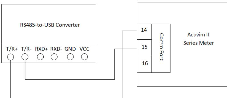
Figure 2-37 RS485-USB Connection to Acuvim II Series Meter
