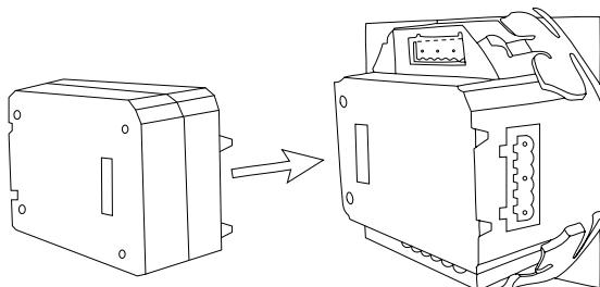
Figure 5-53 AXM-RS485 Installation to Acuvim II Meter
