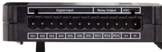
Figure 5-2 AXM-IO1 Module
