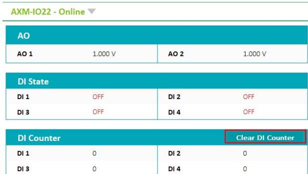
Figure 5-25 Reset DI Counter from Acuvim 2 software
