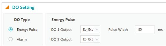
Figure 5-30 Digital Output Configuration from Acuvim 2 Software
