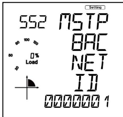
Figure 6-6 System Parameter Setting – S52 MS/TP BACnet ID
