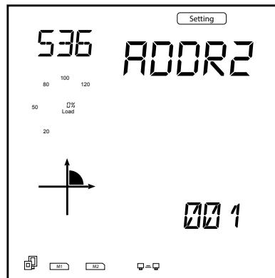
Figure 5-53 Address Setting for AXM-RS485
