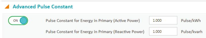
**Figure 5-34 Advanced Pulse Constant Settings from Acuvew 2 Software**
