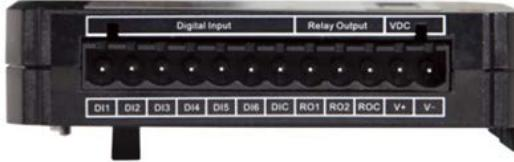
**Figure 5-2 AXM-IO1 Module**
