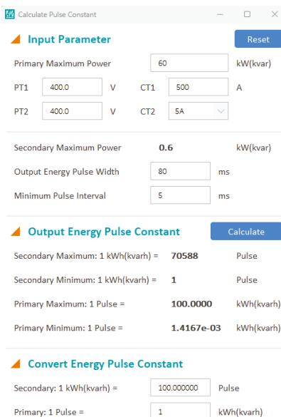
**Figure 5-33 Pulse Constant Calculator from Acuvew 2 Software**
