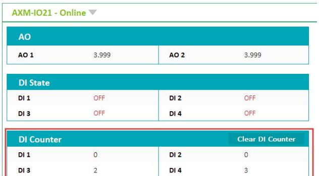
Fig 5-24 Pulse Counter Readings from the Acuvim 2 Software
