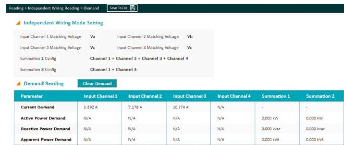
Figure 4-59 Independent Channel Demand Reading
