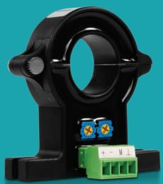
The HAK Series Hall effect DC current sensors provide precision measurements of DC current up to 1000A with a standard 4-20mA or 0-5V output signal for broad compatibility. Featuring a hinged split-core design for fast, easy installation into existing systems, the HAK provides accurate 0.5% measurements for any DC project and is available as either a unidirectional or bi-directional device.
