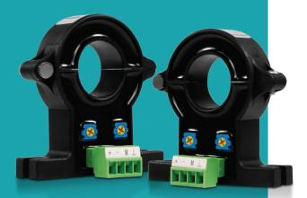
The HAK Series Hall effect DC current sensors provide precision measurements of DC current up to 200A with a standard 4-20mA or 0-5V output signal for broad compatibility. Featuring a hinged split-core design for fast, easy installation into existing systems, the HAK provides accurate 0.5% measurements for any DC project and is available as either a unidirectional or bi-directional device.
