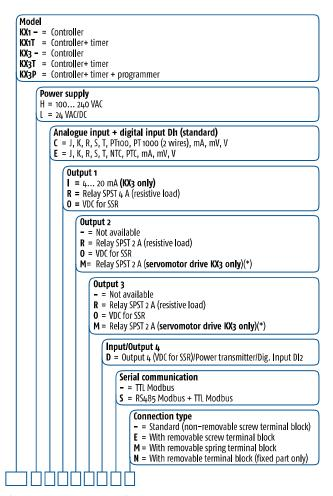
\*: For servomotor drive, both OUT2 and OUT3 codes must be selected as "M".
