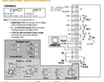
\*: For servomotor drive: OUT2 = open, OUT3 = close.
