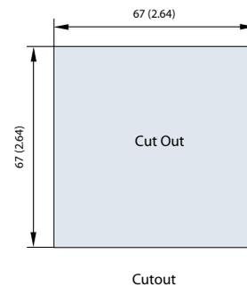
Display Module is designed with flexibility in mind, it can be installed together with the base unit or can be mounted on a panel.\*
