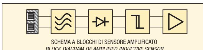
SCHEMA A BLOCCHI DI SENSORE AMPLIFICATO
