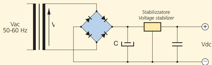
The supply voltage should be adjusted according to the characteristics of the sensor used. It is recommended to use a transformer with secondary voltage Vca lower than the direct voltage Vdc required.
