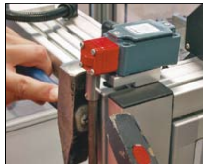
Switch locking (pin provided).
