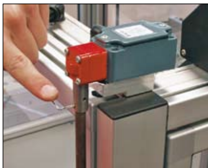
Temporary shaft locking (dowel provided).
