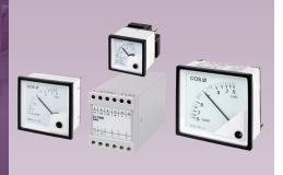
Power factor meters are suitable for the measurement of power factor (cosØ). DIN96 meters are self contained whilst all smaller units are connected to a separate converter unit and calibrated as a complete unit to individual requirements. The converter unit has finger-proof terminal covers and can be remotely DIN rail mounted.
