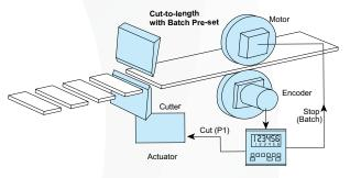
All programming, reset and presetting can be carried out from the front panel.
